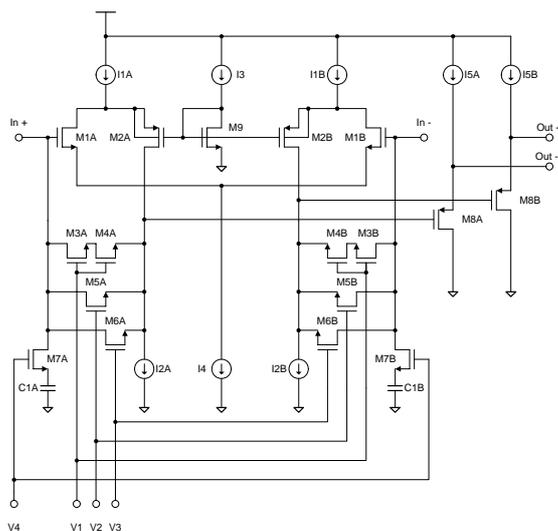
Fig. 11 - Folded cascode differential amplifier cell.
