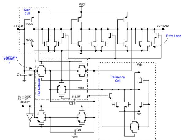
Fig. 9 - Loaded inverter single-ended amplification cell.
