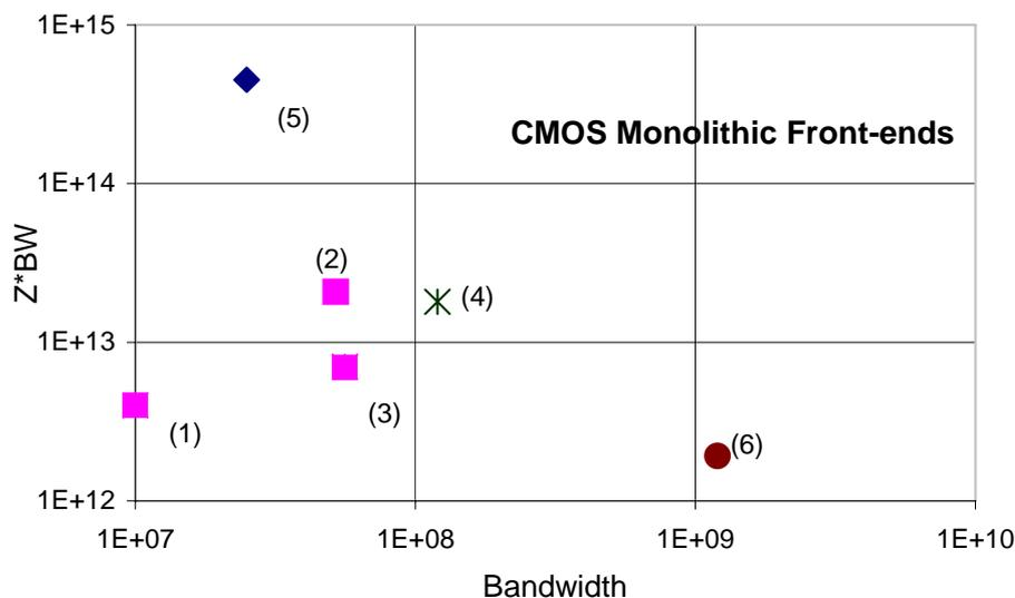
Fig. 13 - Gain\*Bandwidth product versus Bandwidth for several monolithic CMOS front-ends.
