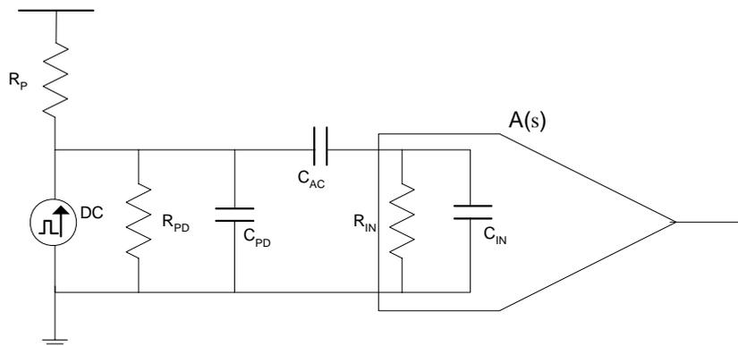
Fig. 6 - Simplified front-end input model.
