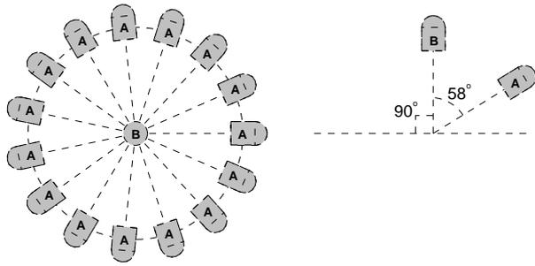
Fig. 4 - IR LED's horizontal distribution (left) and vertical orientation (right).
