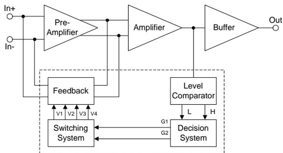
Fig. 10 - Block diagram of a switched gain differential front-end.
