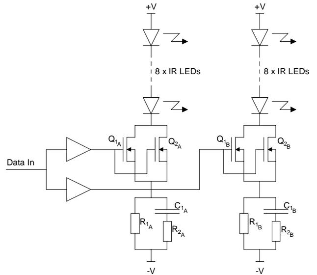
Fig. 5 - Optical emitter simplified circuit.
