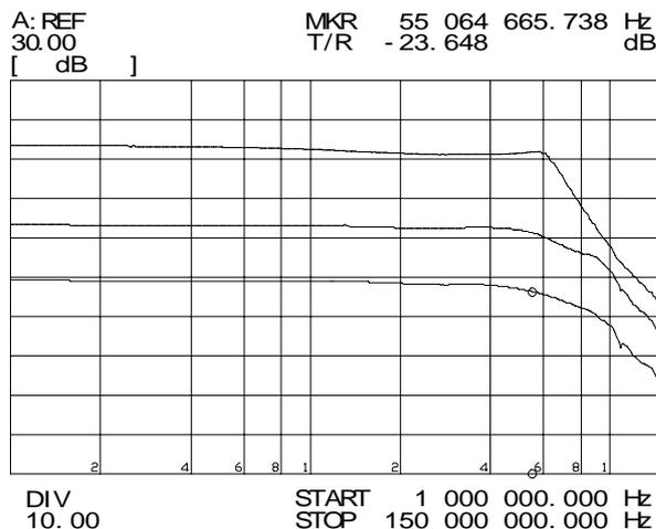
Fig. 12 - Measured transimpedance gains in the folded cascode front-end.
