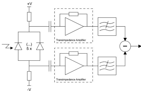
Fig. 7 - Block model of discrete IR front-end.
