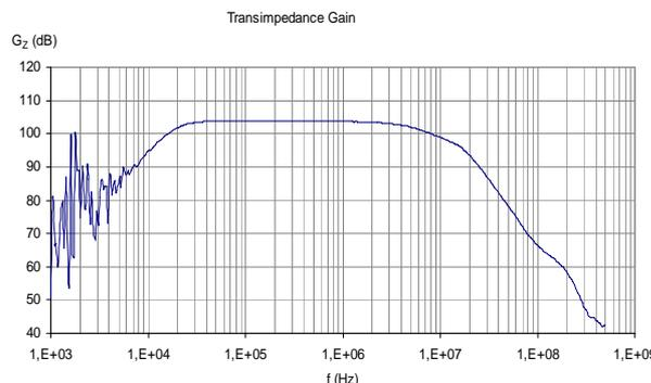
Fig. 8 - Measured transimpedance gain of a discrete low-cost front-end.
