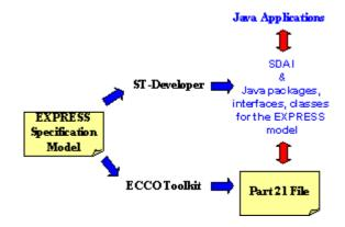
Figure 2. An Object Oriented Implementation Approach for the DDR
