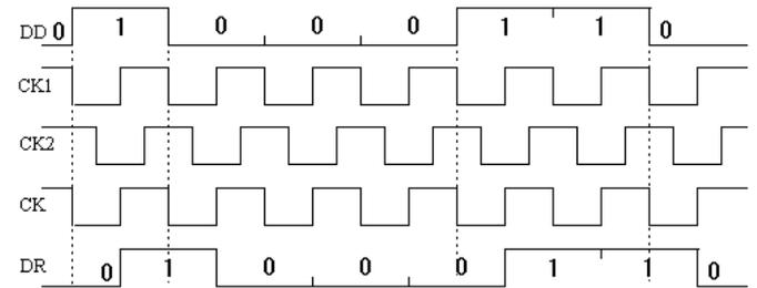
Fig.6 Waveforms at the mixed loop synchronizer
