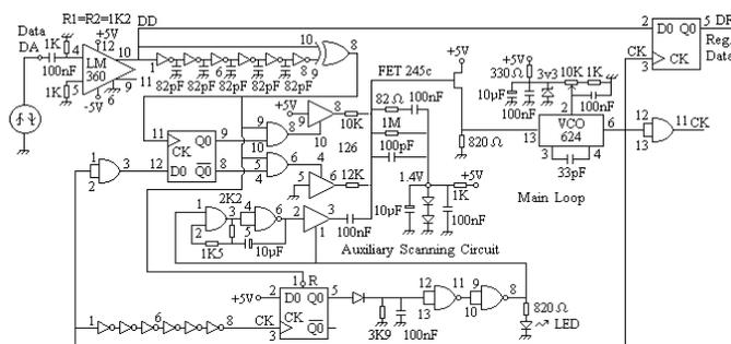
Fig.14 Closed loop synchronizer triggered by input
