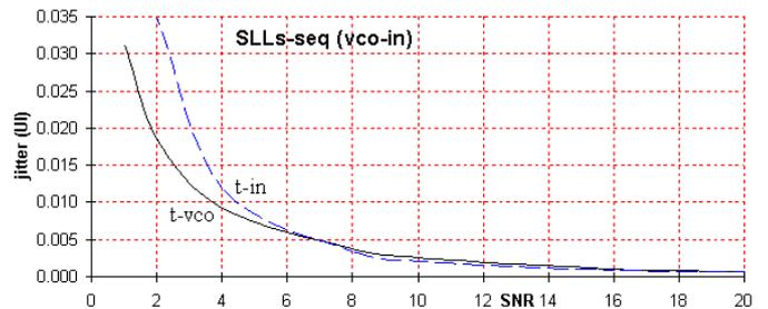
Fig.16 Output jitter UIRMS as function of the input SNR
