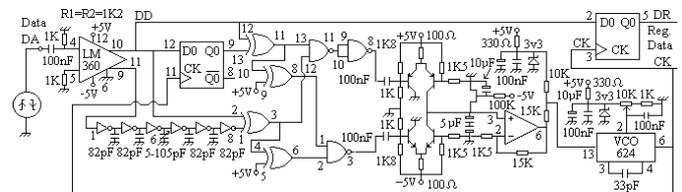
Fig.7 Closed loop synchronizer (triggered by VCO)
