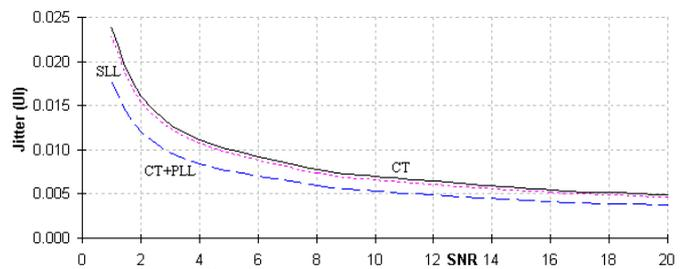
Fig.13 Random error phase (jitter)
