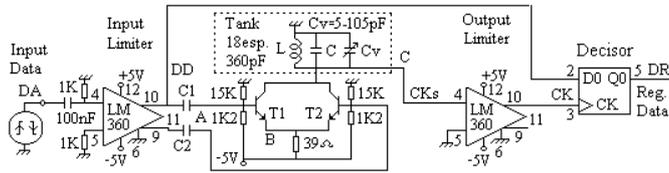
Fig.3 Open loop synchronizer (tank)
