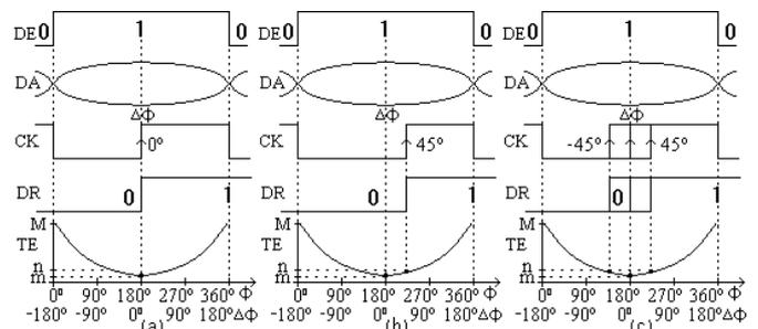
Fig.1 The clock samples the input signal
