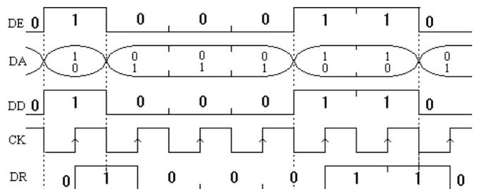
Fig.8 Waveforms at the closed loop synchronizer
