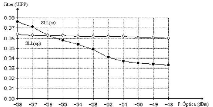
Fig.15 Output jitter as function of the input optical power
