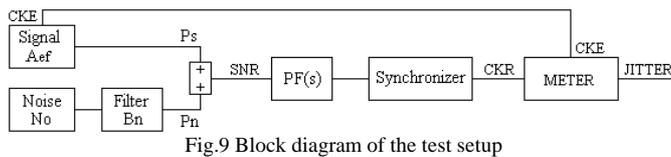
Fig.9 Block diagram of the test setup
