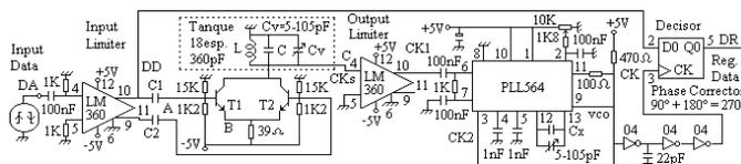
Fig.5 Mixed loop synchronizer (tank + PLL)
