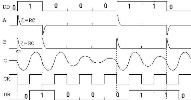
Fig.4 Waveforms at the open loop synchronizer
