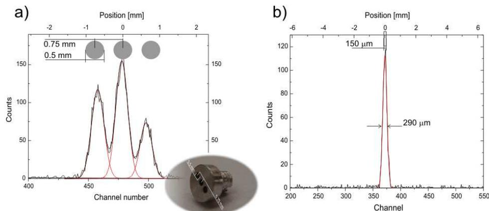
Fig. 1 – a) Al collimator with three 0.5 mm holes with a pitch of 0.75 mm. b) projection of a 0.15 mm slit. The signals are collected from the anodes of the MS-side, the ‘best’ dimension.
