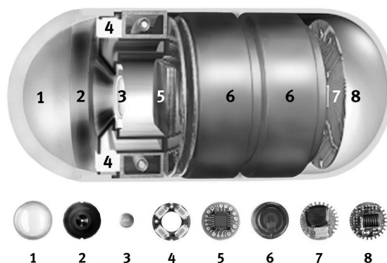
Fig. 1. The wireless endoscopic capsule (1 - Optical dome; 2 - Lens holder; 3 - Lens; 4 - Illuminating LEDs; 5 - CMOS imager; 6 - Battery; 7 - ASIC transmitter; 8 - Antenna).
