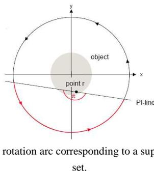
Fig. 5 Focal spot rotation arc corresponding to a super short scan data set.
