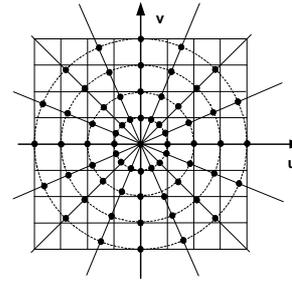
Fig. 4 In Fourier reconstruction, sample points of the 2D Fourier transform of the image are given on a conventional polar grid.
