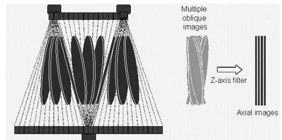
Fig. 7 2D reconstruction over tilted planes and longitudinal filter to obtain axial images (www.impactscan.org).
