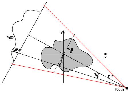
Fig. 2 Object function  $f(x,y)$  and its divergent projection in  $\beta$  direction.
