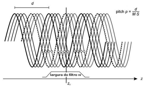
Fig. 6 Interpolation scheme in 180°FMI longitudinal interpolation algorithm [10].
