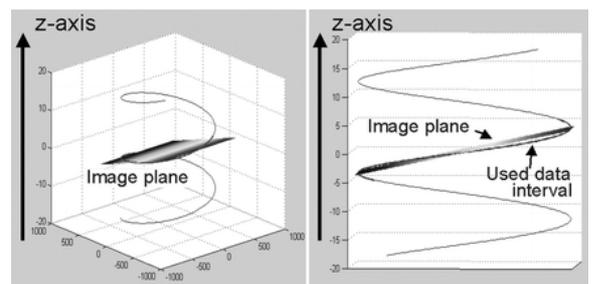
Fig. 8 In ASSR algorithm the image plane is selected in order to minimize the reconstruction error [11].
