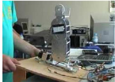
Fig. 28 - Humanoid leg and moving platform where balance experiments based on force were done.
