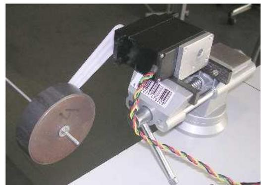
Fig. 6 - Experimental evaluation of the actuator's response using a HITEC HS805BB servomotor.
