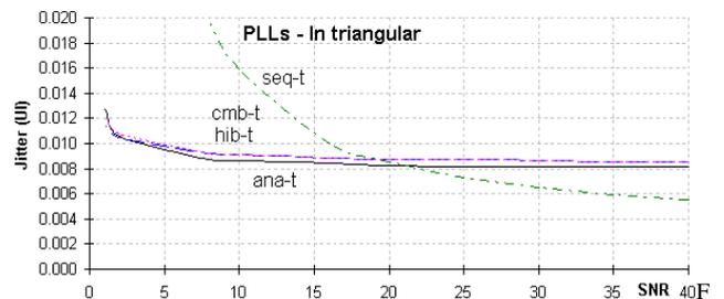
fig.10 Jitter-SNR curves of the four synchronizers (in triangular)
