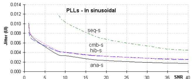
Fig.9 Jitter-SNR curves of the four synchronizers (in sinusoidal)
