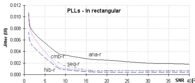
ig.11 Jitter-SNR curves of the four synchronizers (in rectangular)
