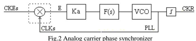
Fig.2 Analog carrier phase synchronizer
