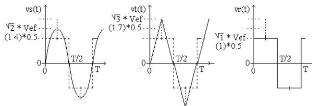
Fig.6 The three input waves: sinusoidal, triangular and rectangular
