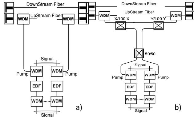
Figure 4.a) Simple Remote node pump topology and b) double power splitter pump topology [10].
