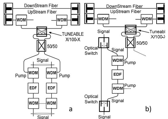
Figure 7.a) Tunable Power Splitter pump topology and b) reconfigurable modules pump topology [12].
