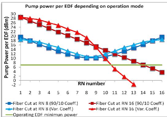
Figure 6. Comparison of variable and 90/10 power couplers for different states of the network [11].
