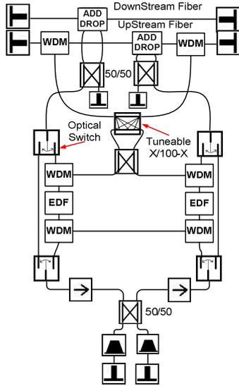
Figure 12: Remote Node topology considering the better pump and signal topologies providing full reconfigurability of the network [10].
