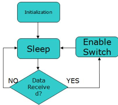
Figure 14. Schematic of the harvesting and control module and the micro controller states.
