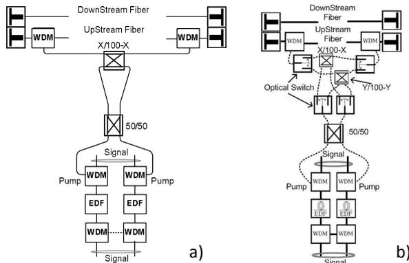
Figure 5.a) Single power coupler pump topology and b) optical switching [10].
