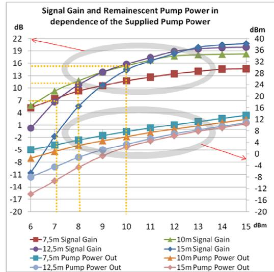
Figure 13: Signal Gain and pump reminiscent in function of the input pump power and EDF length.
