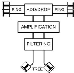
Figure 3. Remote Node main structure [10].
