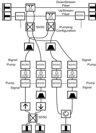
Figure 10: Remote Node topology based on OADM thin filters [10].
