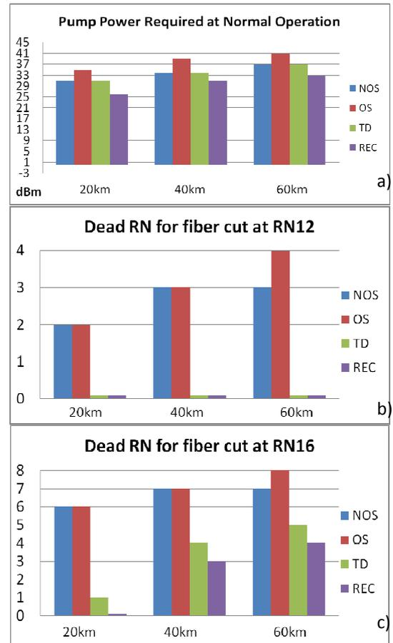
Figure 15. Results of the SARDANA network simulation for 20, 40 and 60km of ring length. a) Pump power required to the CO, b) number of dead RNs (RN not supplied with enough pump power) for fiber cut at RN12, c) number of dead RNs for fiber cut at RN16.
