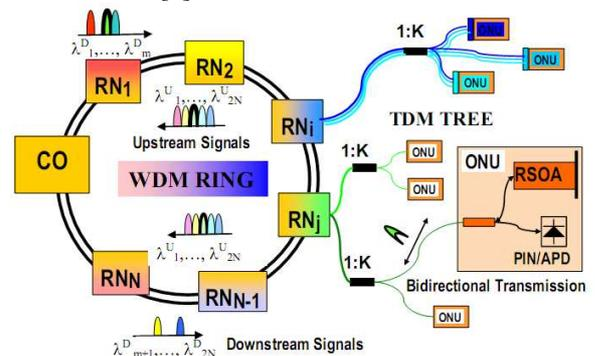
Figure 2. SARDANA network architecture [3].
