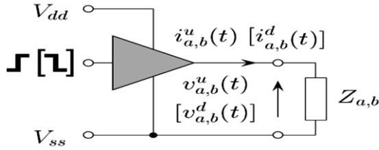
Fig. 12: Simulation setup for the generation of the identification signals for the weight coefficients  $W_1$  and  $W_2$ . The current and voltage data are recorded while the driver is loaded by two different loads and is driven to perform an up and down state transitions [4].
