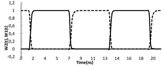
Fig. 13: Weighting functions  $w_1$  (straight line) and  $w_2$  (dotted line) that control the switching between  $f_1$  and  $f_2$ .
