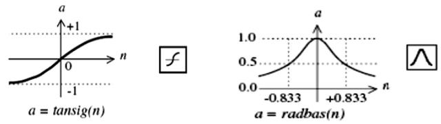
Fig. 4: Tan-Sigmoid and Radial Basis activation functions used in ANN are bounded in output amplitude.
