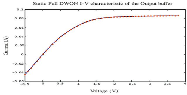
Fig. 10: Function fit for submodel  $f_2$ . Transistor-level (straight line) and feed-forward ANN model (dotted line).
