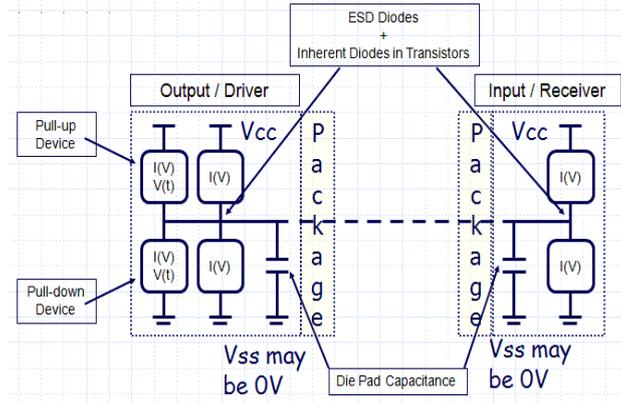
Fig. 1: Key portions of an IBIS driver and receiver model
