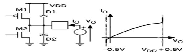
Fig. 7: Simulation setup for the steady state identification signals for submodels. The clamp diodes start to conduct as the output voltage exceeds the supply voltage bounds.
