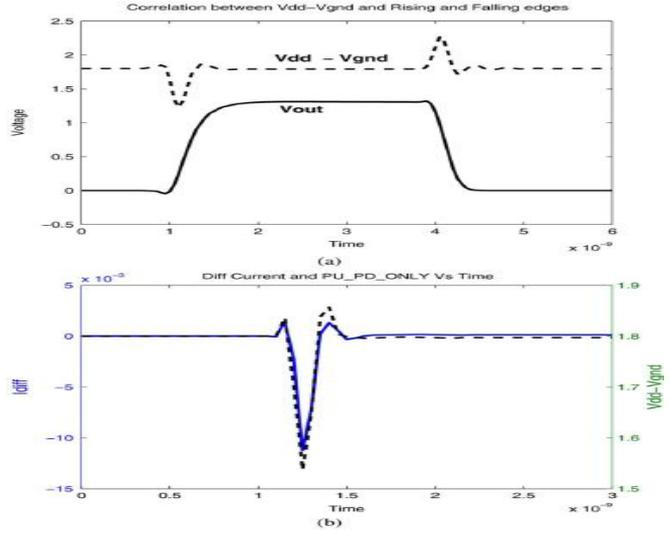
Fig. 2. Power drop and ground bounce correlate with the switching of the buffer (a). There is a high correlation between the difference in current (solid line) at the  $V_{DD}$  pin between the transistor level model and the behavioral (IBIS) model and  $V(Pwr-Gnd)$  (dashed line) (b).
