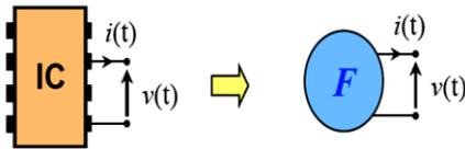
Fig. 3: The observed electrical behavior IC driver circuit is reproduced by a suitable  $F[\cdot]$  mathematical relation.
