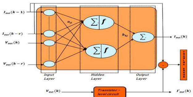
Fig. 11: Scheme used in the training process of the NARX model.
