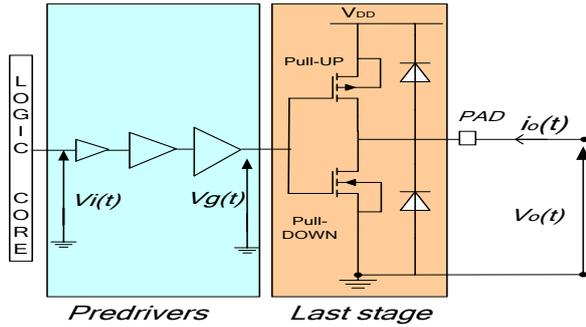
Fig. 5: Generic multistage driver and its relevant electric variables.
