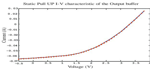
Fig. 9: Function fit for submodel  $f_1$ : Transistor-level (straight line) and feed-forward ANN model (dotted line).
