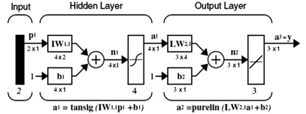
Fig. 6: Structure of feed-forward ANN (source: MATLAB).
