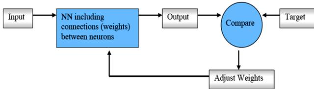
Fig. 8: The weight and bias parameters are iteratively adjusted during the training process (source: MATLAB).
