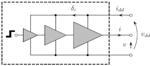
Fig. 15: General structure of a driver circuit and its relevant (output and power supply) port electric variables [8].
