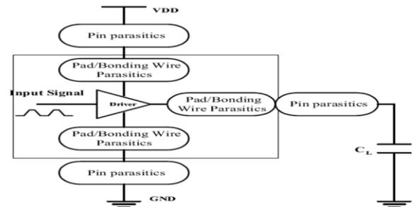
Fig. 14: Block diagram of the chip-package interface.
