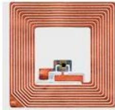
Figure 8: HF RFID tag example (13.54MHz) [11]
