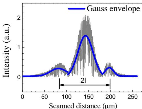
Fig. 4 Aproximation envelopes for the interference pattern, where  $l$  is the difference of paths travelled by the beam in the interferometer.
