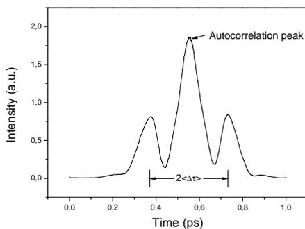
Fig.1 Interferogram envelope example for non-mode coupled devices.
