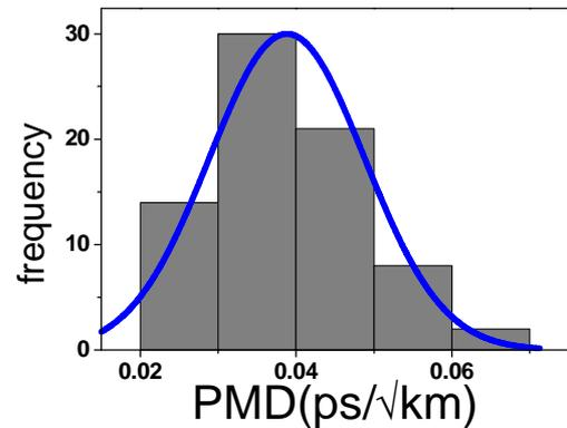
Fig. 5 Histogram of determined PMD values for Reel 1 in a 32 days time interval, with its normal representation.
