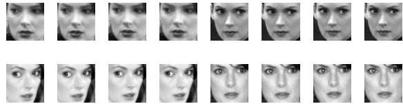
Fig. 5 - Extended database: 1 original image gives 4 new images ( p = q = 2 )
