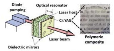
Proof of the concept of possibility to develop a new type of Q-switched laser materials
