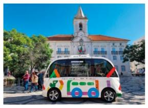
autonomous vehicle to demonstrate that it is possible to control the movement of the vehicle through a smart city. This mechanism has been extended with sensors and intelligent algorithms to detect the presence of people crossing the road: from the lamppost, a "stop" message is sent to the vehicle, the vehicle stops and people can cross the road. This mechanism has been demonstrated and tested in the road (<u>https://www.</u> youtube.com/watch?v=3q-LblHoZhY).
