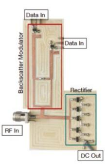
Our work presents a system composed of a backscatter modulator at 2.45 GHz with data rates up to gigabit which is shown in Figure 1. Moreover, a rectifier that is capable of converting the RF signal into DC power also composes the system. The proposed system enables low power consumption, while maintaining a high modulation bandwidth (16-QAM).
