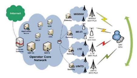
proposed a seamless mobility architecture with QoS support in heterogeneous wireless access environments. The proposed architecture integrates an extended version of IEEE 802.21 framework with QoS support, as well as an advanced mobility manager integrated with the Mobile IP (MIP) mobility
