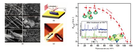
Piezoelectricity, the ability of noncentrosymmetric materials to produce mechanical stress/strain under an electric field or charge/voltage under a mechanical force, is widely used in many areas, e.g. in medical ultrasound transducers and filters for mobile phones. Until recently, only inorganic piezoelectrics (such as PZT or LiNbO<sub>3</sub>) have been used based on their high piezoelectric coefficients. In view
