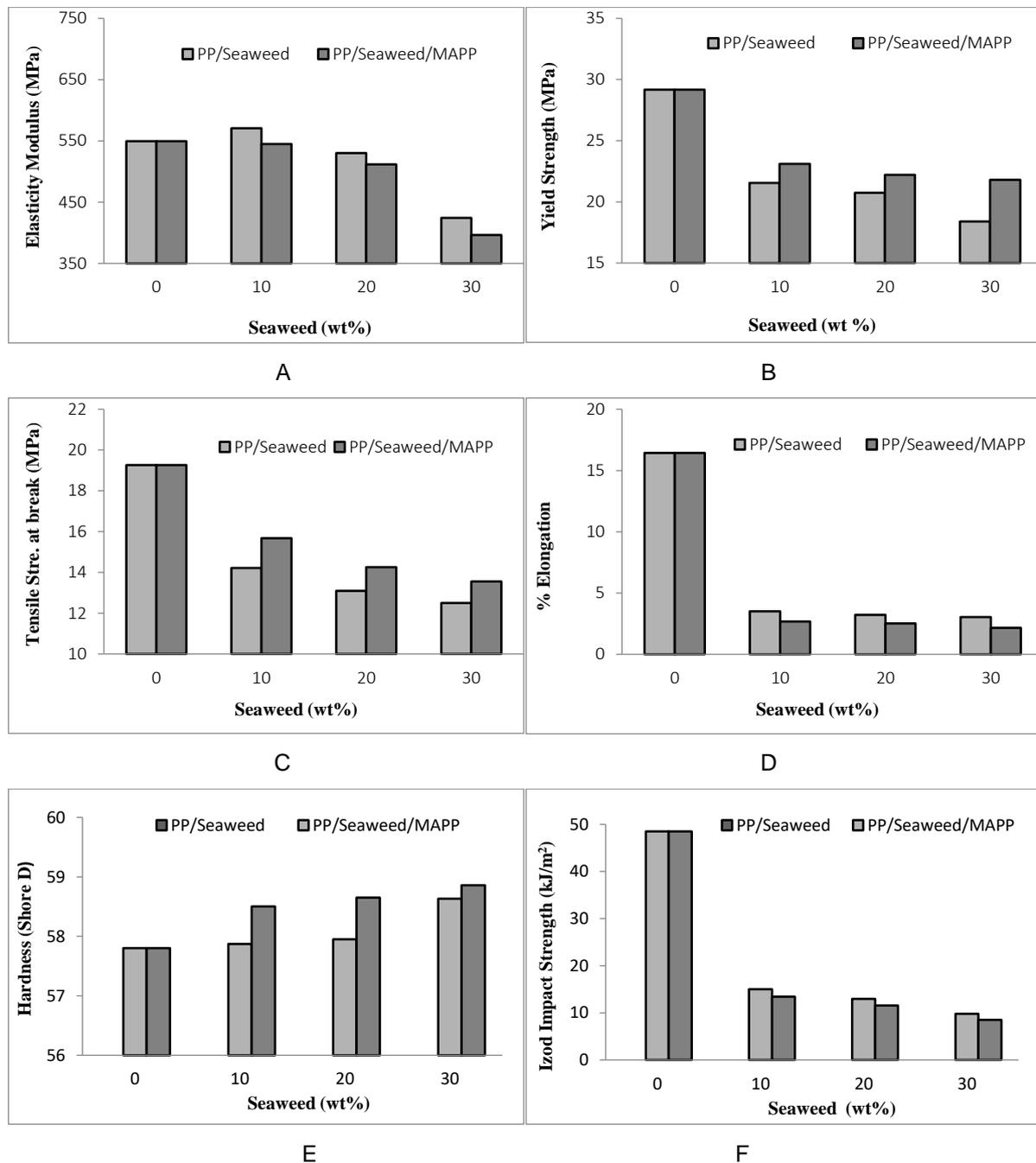
Figure 2. Mechanical properties of PP/SW/MAPP polymer composites.
