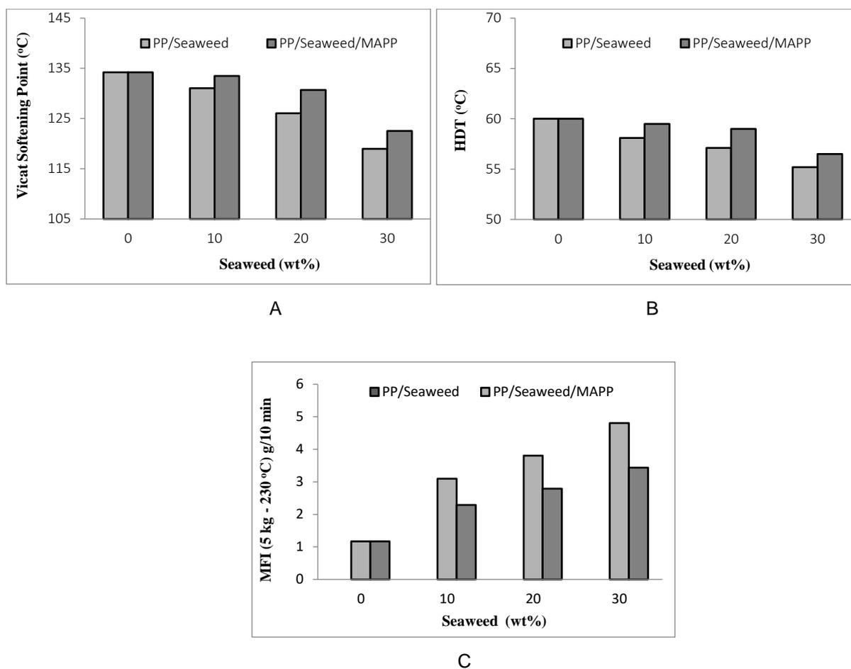
Figure 3. Physical properties of PP/SW/MAPP polymer composites.
