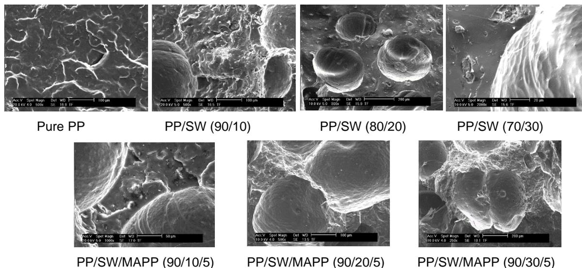
Figure 4. SEM photographs of PP/SW/MAPP polymer composites.
