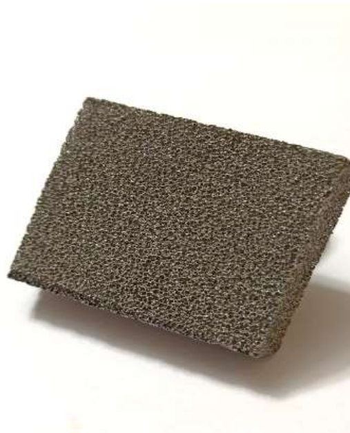
Figure 2. Aluminum foam of 86% porosity.
