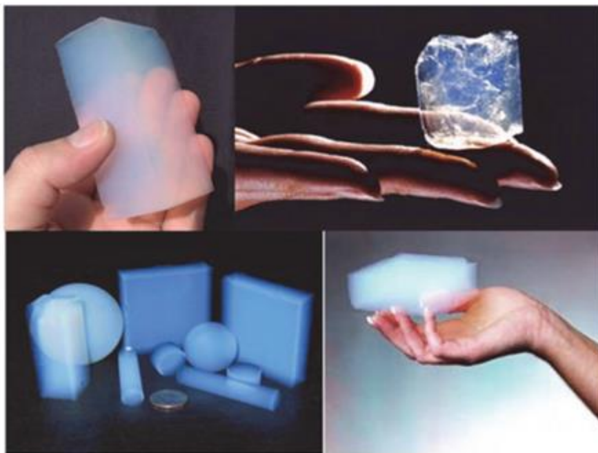
Figure 11. Airgel and silica-airgel specimens that can efficiently spotless against water, sea-ocean, and ground oil spills.
