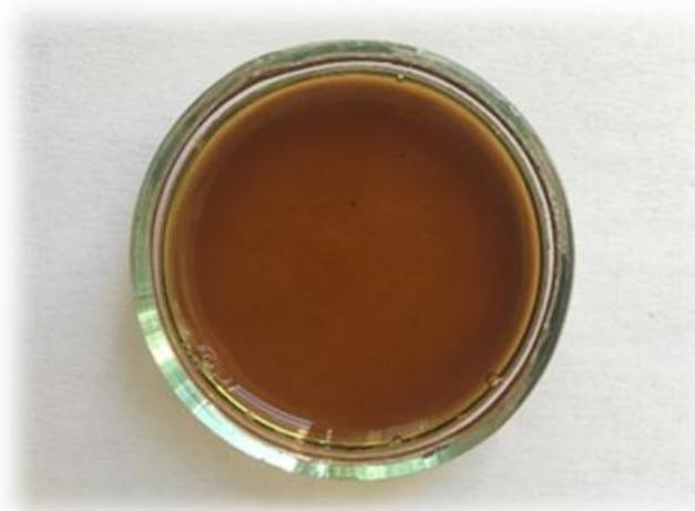
Figure 1. Synthesized graphene oxide slurry by Hummer's method.
