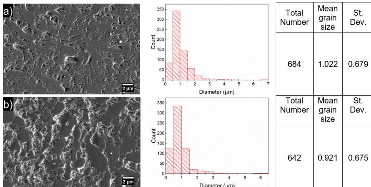
Figure 4. The micrographs of alumina samples a) pure alumina, b) with addition of waste alumina (20 dwb. %) and their corresponding grain size distribution from image analysis of SEM micrographs.
