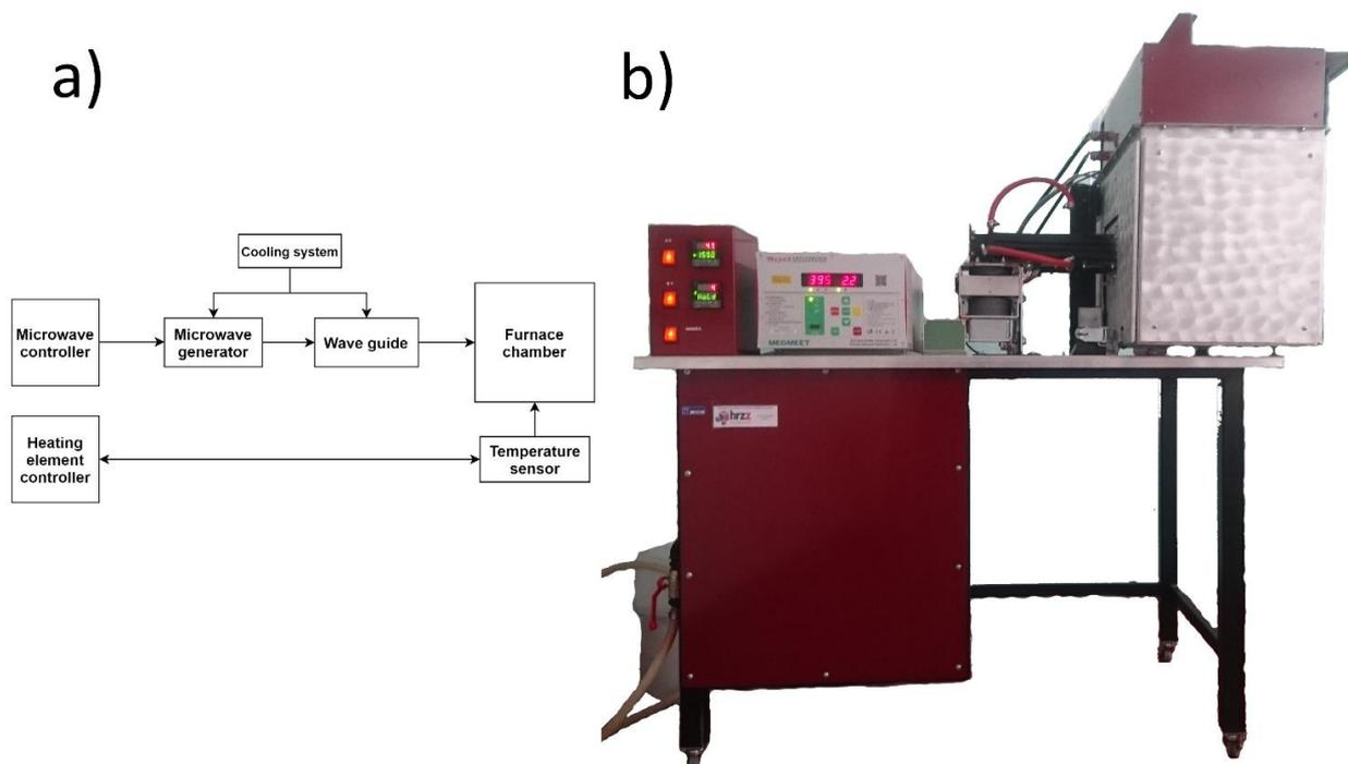
Figure 2. The schematic diagram (a) and photograph of the hybrid microwave furnace (b).
