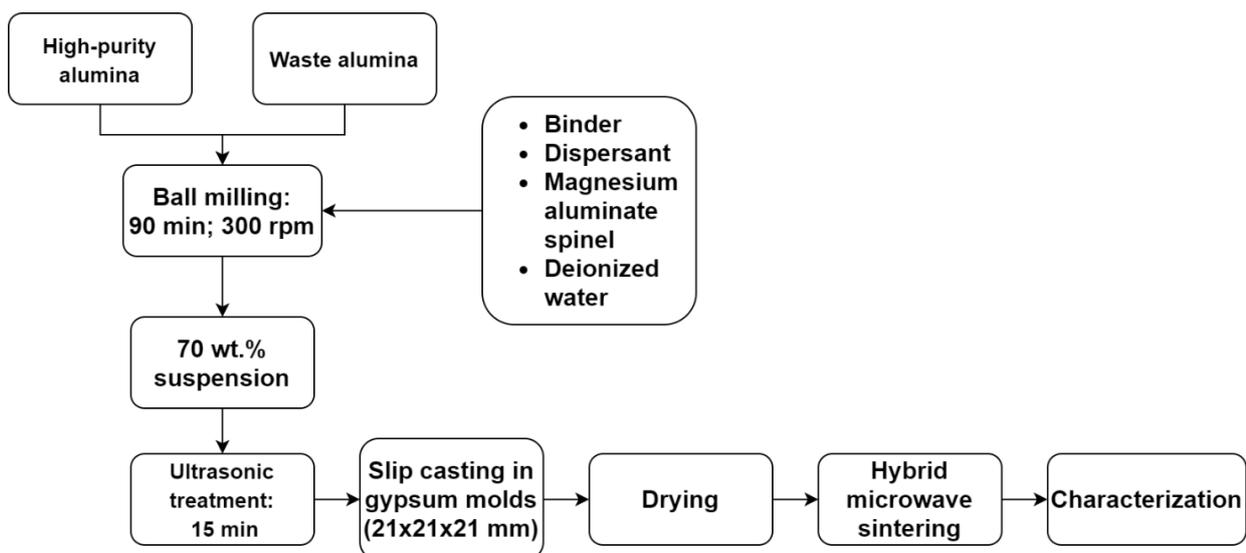
Figure 1. Process flow chart for sample preparation.
