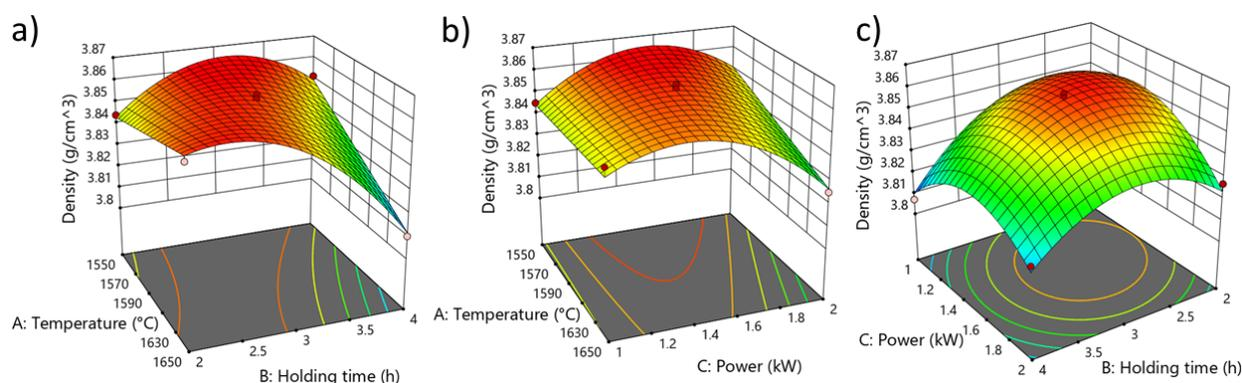
Figure 3. a-c) represents the response surface plots (3D) showing the effects of sintering parameters on the response density of sintered samples: a) fixed value of input power at 1.5 kW, b) fixed value of holding time at 3h, c) fixed value of sintering temperature at 1600 °C.
