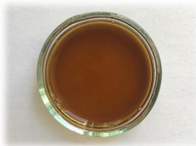
Figure 1. Synthesized graphene oxide slurry by Hummer's method.
