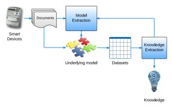
Fig. 5. Architecture of the knowledge extraction platform.
