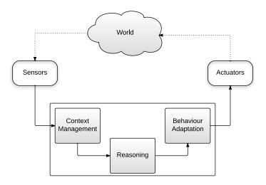
Fig. 1. Conceptual Architecture of a Smart Environment
